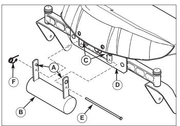
Figure 1. Install Counter Weight
